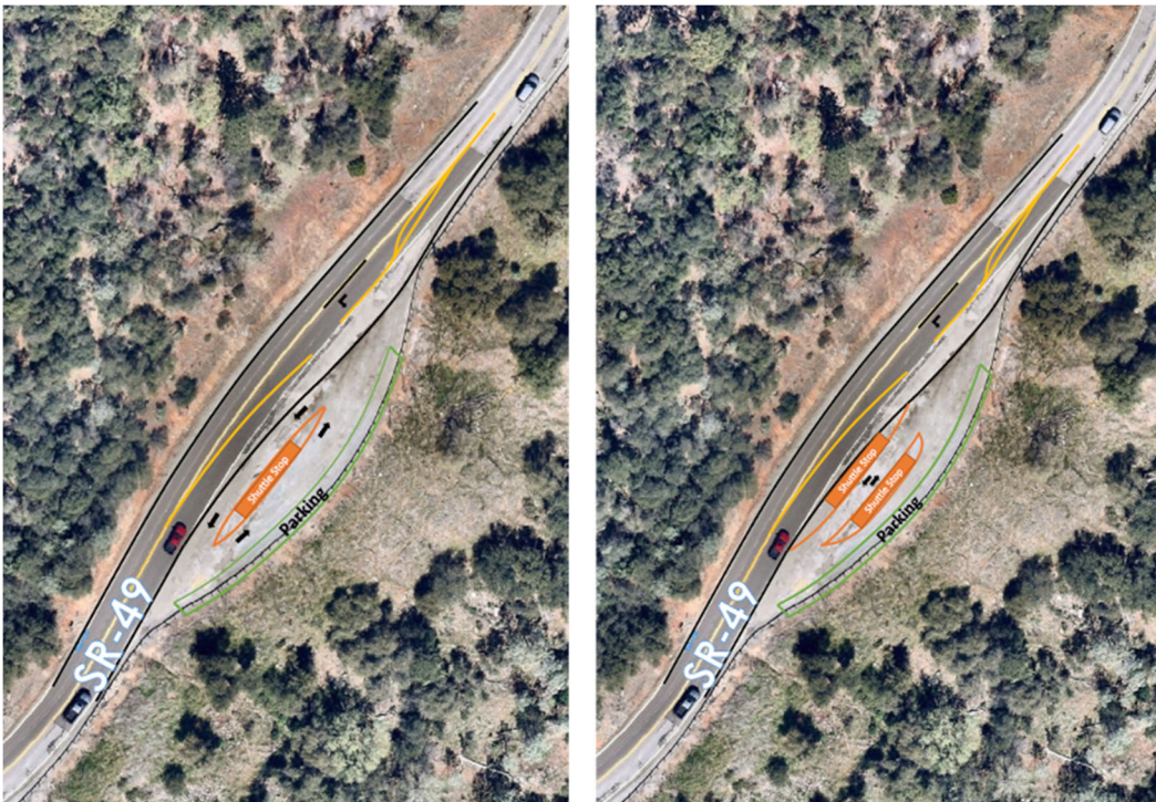
FIGURE 60: CONCEPTUAL DESIGNS FOR SHUTTLE STOP EAST OF ROBBIE POINT
