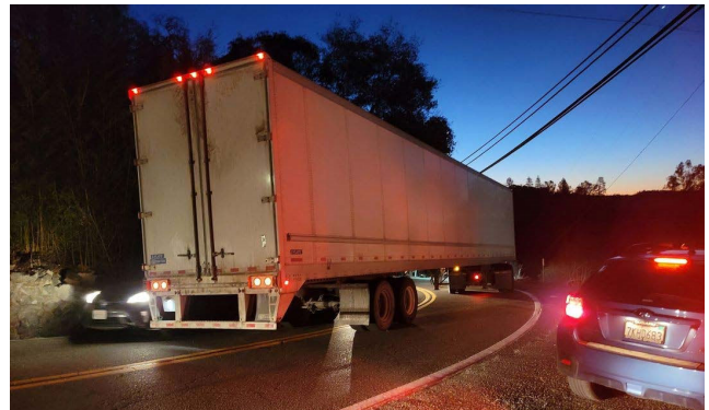
FIGURE 53: OVERSIZE TRUCK TRACKING INTO OPPOSITE LANE
